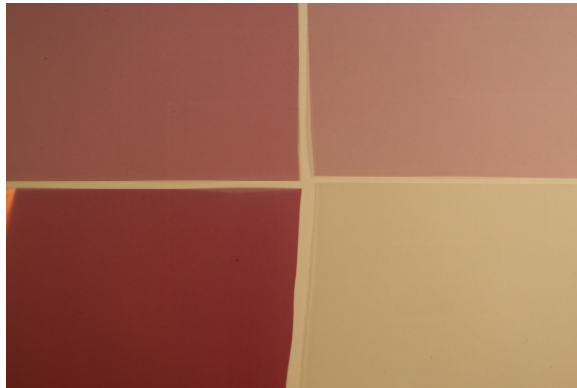
Figure 4.5. Thin (10–50 nm) and homogeneous P3HT layers applied by reverse gravure coating onto a 12 cm wide polyester film are shown.
