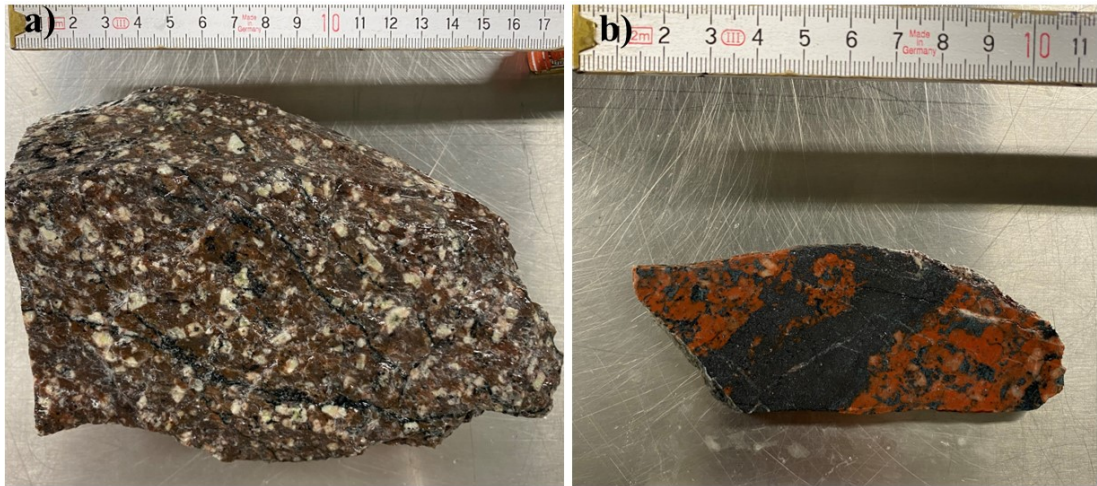
Fig. 10. (a) Hand sample of red quartz-bearing porphyry (from crosscut 335, level 1194). (b) Sample of red, altered quartz-bearing porphyry, showing interaction with ore, sampled at their contact (from crosscut 173, level 1165).
