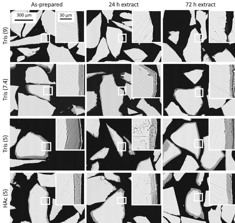
Fig. 3. SEM images of S53P4 particles immersed in the four as-prepared solutions and their 24 and 72 h extracts for 120 h.
