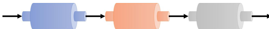
Figure 6. A cascade reactor setup with three reactors coupled in series. The solution flows from left to right.
