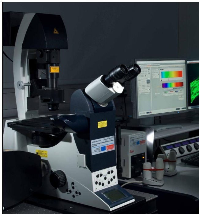
Figure 9. Basic confocal instrument setup (Warwick University, 2017).
