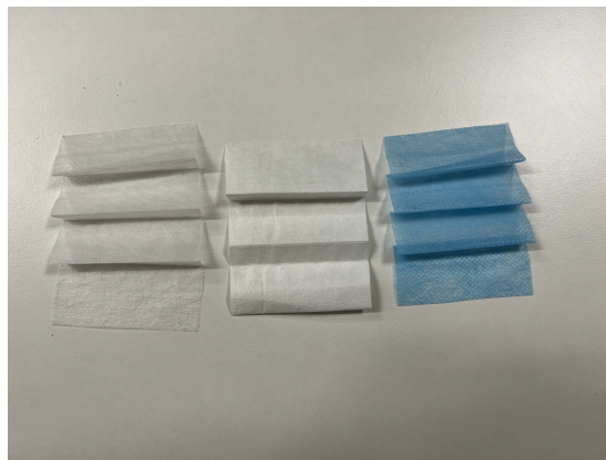
Figure 2: Skin-friendly layer (left), Filter layer (middle), Protective layer (right)
