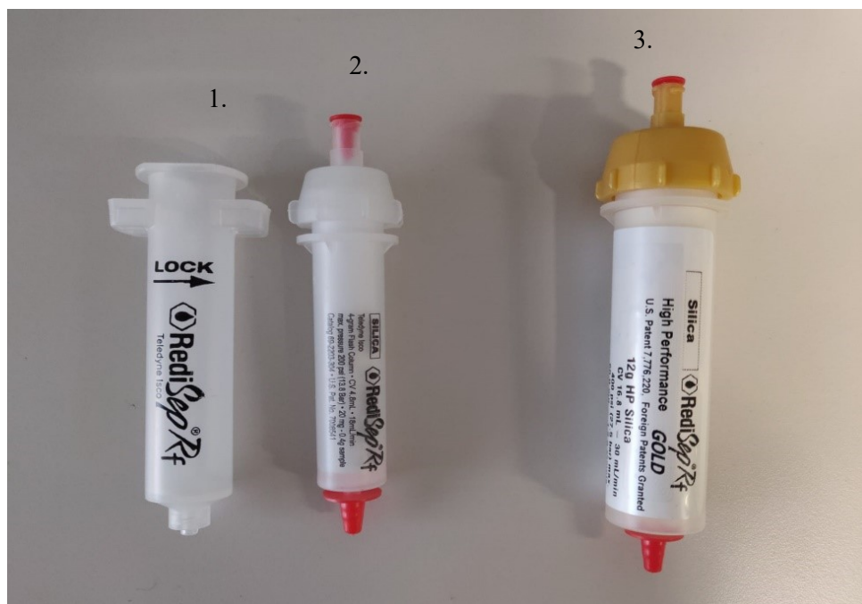
Figure 9 Sample tube (1.), 4 g silica column (2.) and 12 g silica gold column (3.) used for the automated normal-phase flash chromatography.
