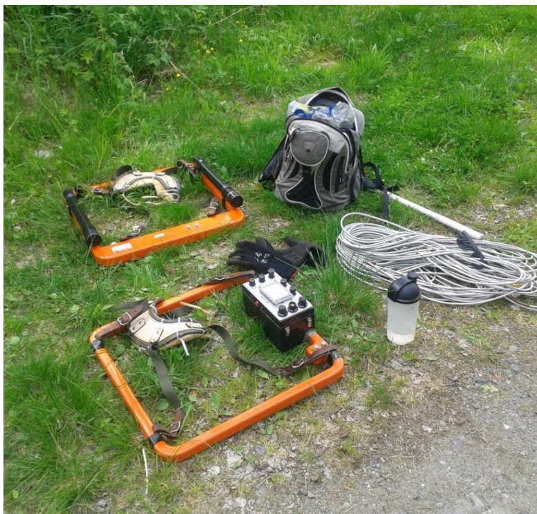
Figure 7. The Slingram equipment disassembled on the ground. The orange transmitter and receiver lie in the back and in the front, respectively. The 60 m cable lies to the right.
