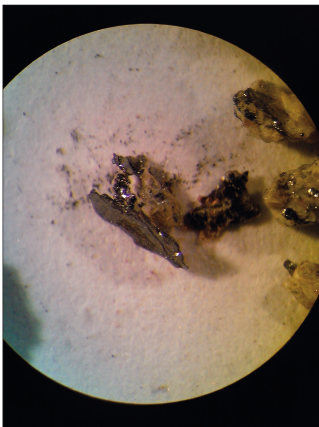
Figure 3. Distinct graphite flakes after fragmentation in a selFrag device (sample 300266.3), fraction 0.5–1 mm. The big flake is approximately 1 mm in length.
