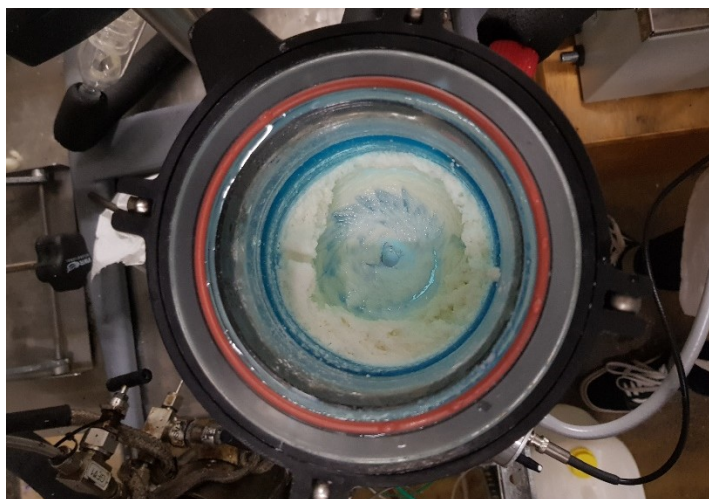
Figure 12 - An image of the solidification in the discontinued experiment at 30 °C. Picture taken from above of the batch reactor
