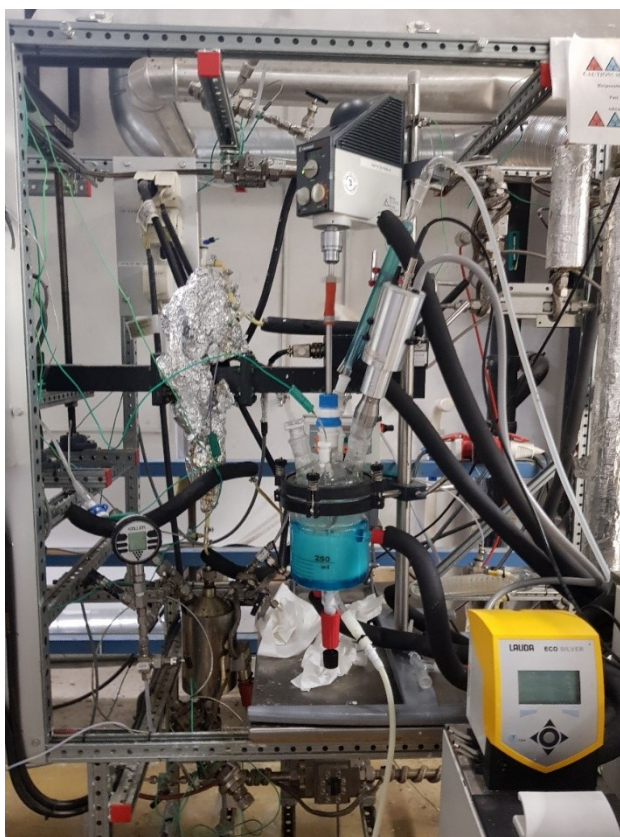
Figure Appendix I 4 - Image of the isothermal batch reactor system with the ultrasound probe in use
