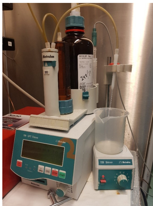
Figure Appendix I 2 - Analysis equipment for oxirane number titrations with perchloric acid
