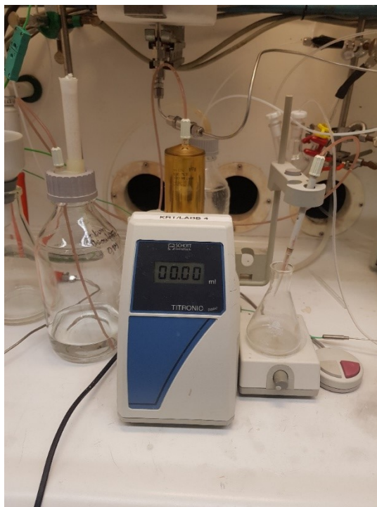
Figure Appendix I 1 - Analysis equipment for iodine value titrations with sodium thiosulphate
