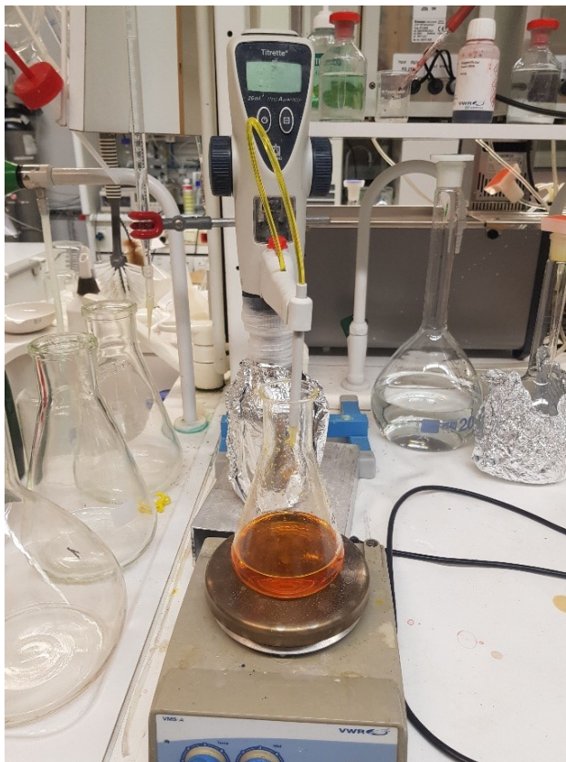
Figure Appendix I 3 - Analysis equipment for hydrogen peroxide titrations with ammonium cerium sulfate
