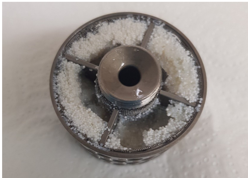
Figure 6 – Novozym® 435 in the SpinChem® RBR after using as a rotating catalyst bed
