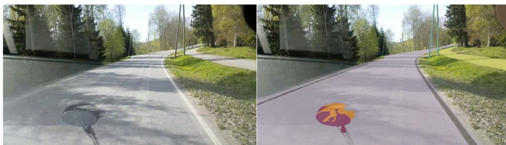
Figure 6. An example of how objects on the dashboard can affect computer vision when no polarisation filter is placed in front of the camera lens.
