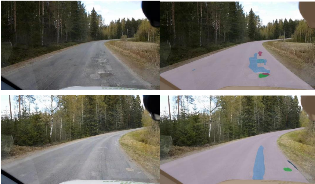
Figure 14. Computer vision: moderate hole. Person 1: no hole detected (2 instances, marked in green in the segmentation image).
