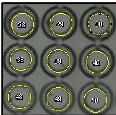
Figure 42. Circular ROIs for wells – These ROIs were drawn for the image data on ImageJ. This way changes occurring in these ROIs can be processed by ImageJ as zebrafish movement.
