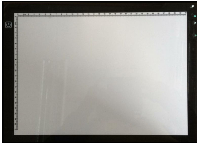
Figure 12. Planar White LED Light Source – This is LED copy board A4. The size of light source was 36 cm x 24cm and height 5mm. The entire cardboard box easily fitted onto the surface of this light source.
