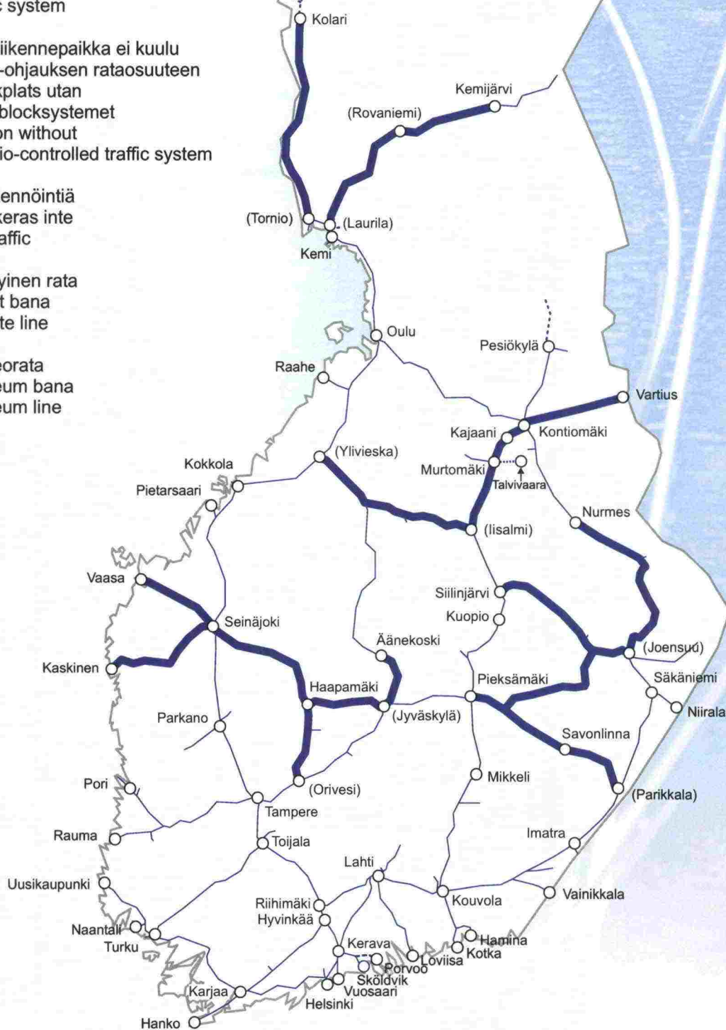
Figure 4. Lines with radio-controlled traffic system.
