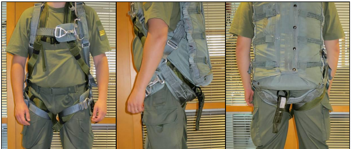
Figure 18. Emergency parachute worn with Airsafe Sweden ab's Cabin Safety Harness CSH 2-1560. The connection point for the attachment strap is visible at the back below the parachute container
