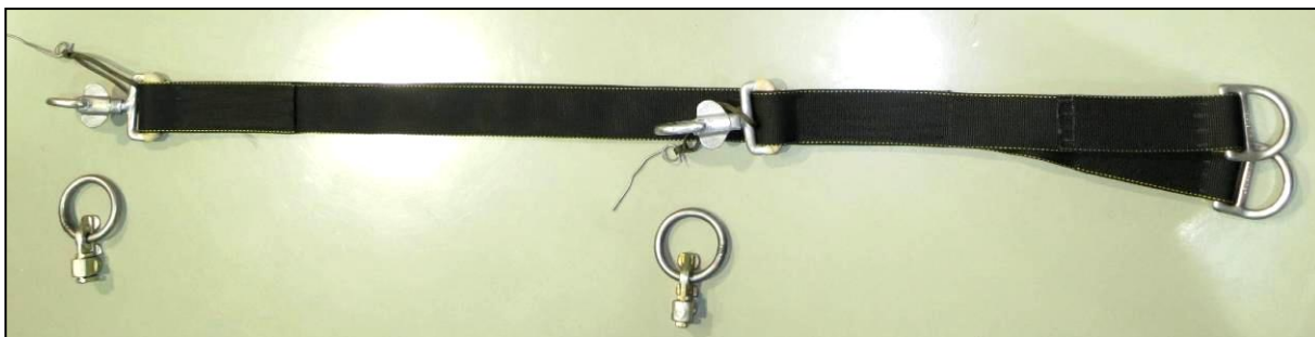
Figure 12. The PASI-1 anchor line and two separate Quick Release Cargo Rings, commonly used in transport aircraft. See list of components and their specifications in Table 10 (Appendix 4). The total length of PASI-1 is approximately 1 metre.
