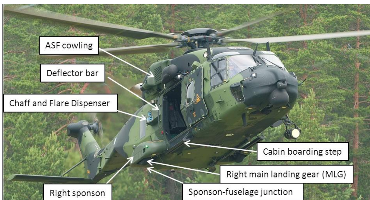
Figure 6. NH90 TTH TFIA IOC+ (tail number NH-215) in hovering flight. The right cabin door is open with the black Parachuting Kit deflector bar installed aft of the door on the outside. Some other test relevant items are also pointed out
