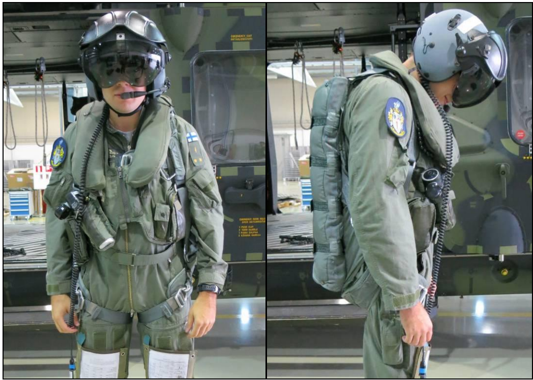
Figure 17. Helmet Integrated System Ltd's Alpha-helmet (P/N: SCA0079946), Pioneer Aerospace Corporation's emergency parachute (P/N 2711-519) and Beaufort Ltd's Helicopter Flight Jacket (P/N: A356800A01/2/3) worn by a crew member
