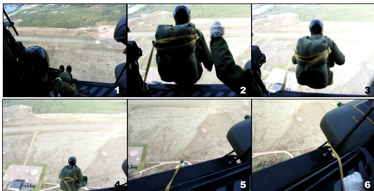
Figure 24. A jumper's exit at 60 KIAS from a seated position. In the readiness position (step 1) the jumper was sitting on the cabin floor facing directly to the side. The feet were hanging outside and hands beside thighs on the door edge. After exit the static line first contacted the middle of the boarding step, then stabilised against the bar between the step and the sponson as seen in step #6 on the bottom right
