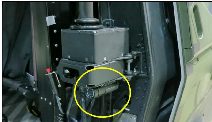
Figure 15. Contour HD 1080p digital video camera, facing towards the tail of the helicopter, installed with cable ties below the Winch Man Trim (WTR) unit
