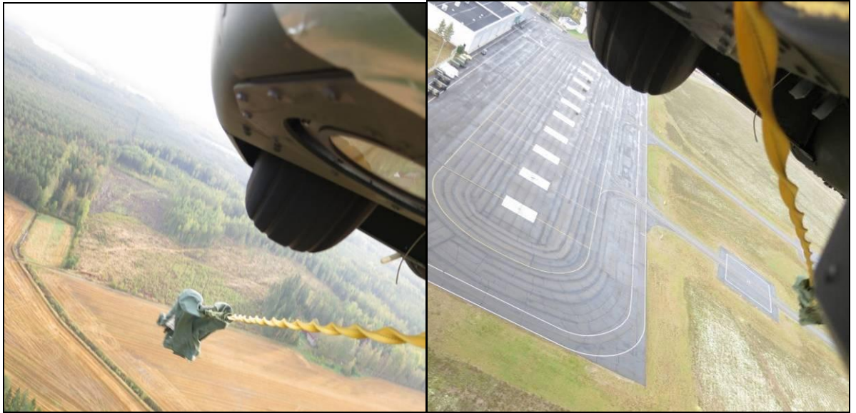
Figure 21. One static line + D-bag below the sponson at 40–50 KIAS with PASI-1. On the left the situation with slip ball on the left (side slipping to the left) and on the right with slip ball on the right (side slipping to the right)
