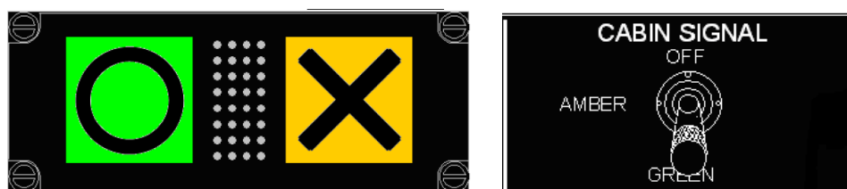
Figure 8. Parachuting Drop Light (PDL) panel is on the left and its control panel (in cockpit) on the right. The green (“JUMP”) and yellow (“STAND-BY”/ “STOP”) lights have been symbol coded to be readily readable even if operating with NVGs. [14, p. 13] When approaching the jump site the cockpit crew selects CABIN SIGNAL switch to AMBER illuminating amber light on the cabin PDL, meaning “STAND-BY” (or “STOP/ABORT” if lit after GREEN light). At the exit point GREEN position is selected, which illuminates green light on PDL and initiates an audio tone
