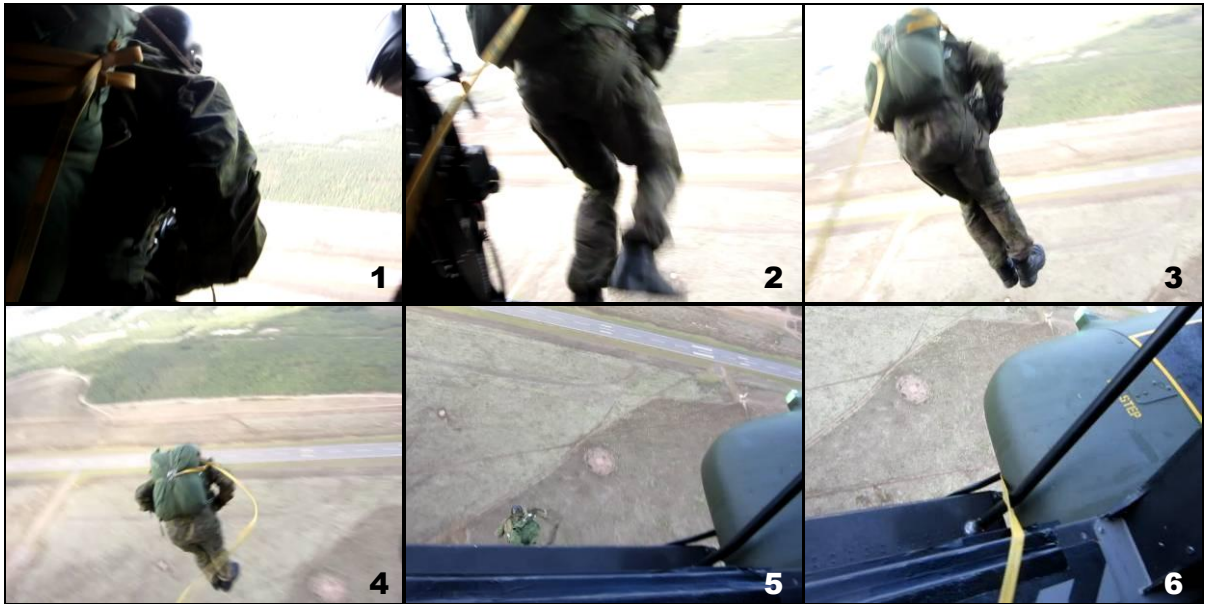
Figure 25. A jumper's exit at 50 KIAS from a standing position. In the readiness position (step 1) the jumper was standing on the left side of the door left foot forward. After jump the static line stabilised against the bar between the step and the sponson, contacting also the deflector bar
