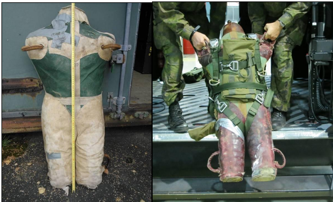
Figure 16. The parachutist test dummies used by the FDF. On the right a dummy is shown at the cabin door with the T-10 harness on. Two people are normally required to handle the 100 kg dummy and push it from the door
